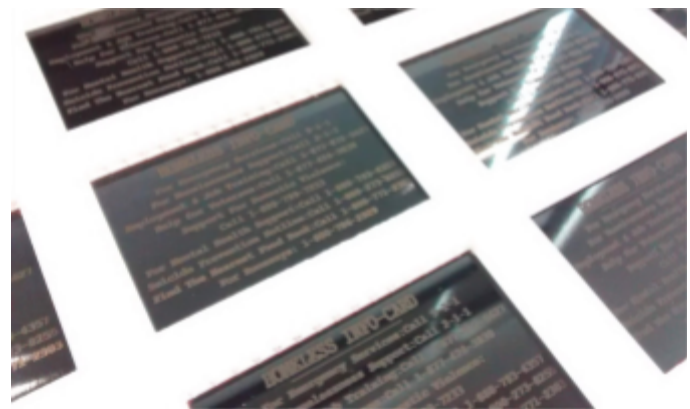
Image 3. Laser engraved information cards for homeless people. Info cards were engraved on thin metal sheets for durability and weather resistance.
